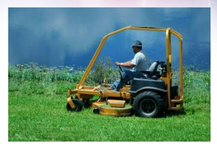
This lawnmower has a roll bar to protect the operator from rolling over on an incline. These mowers also have seat belts that must be used for additional protection.
